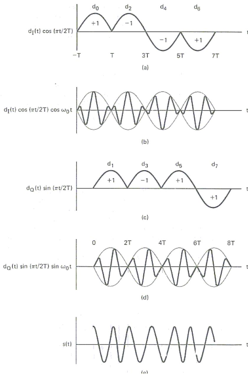
The MSK modulation makes the phase change linear and limited to  $\pm (\pi/2)$  over a bit interval  $T$ . This enables MSK to provide a significant improvement over QPSK. Because of the effect of the linear phase change, the power spectral density has low side lobes that help to control adjacent-channel interference. However the main lobe becomes wider than the quadrature shift keying.
