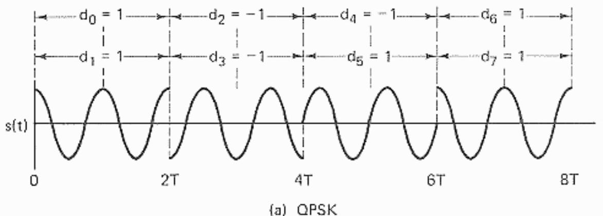
If a QPSK modulated signal undergoes filtering to reduce the spectral side lobes, the resulting waveform will no longer have a constant envelope and in fact, the occasional  $180^\circ$  shifts in phase will cause the envelope to go to zero momentarily.
