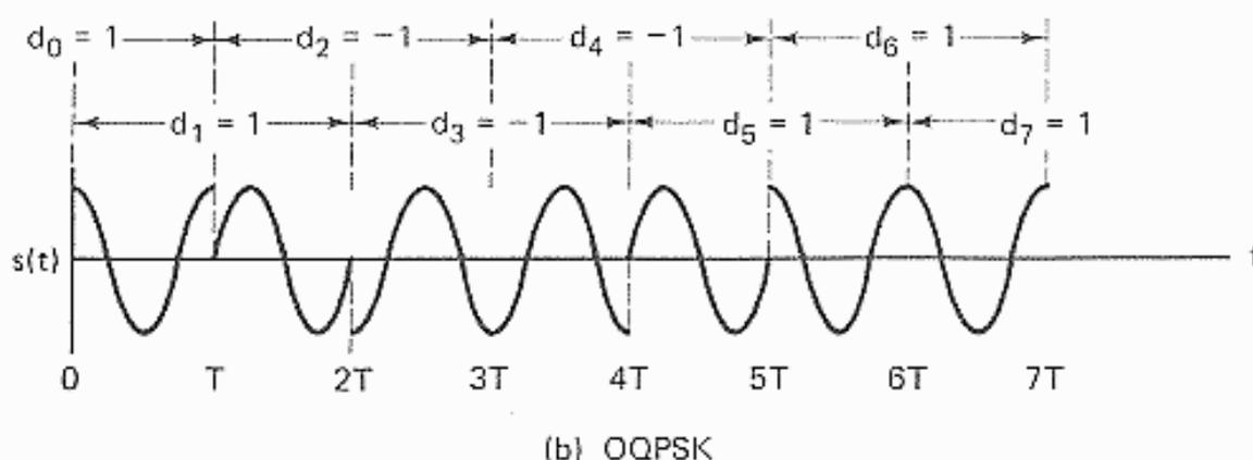
When an OQPSK signal undergoes bandlimiting, the resulting intersymbol interference causes the envelop to droop slightly to the region of  $\pm 90^\circ$  phase transition, but since the phase transitions of  $180^\circ$  have been avoided in OQPSK, the envelop will never go to zero as it does in QPSK.
