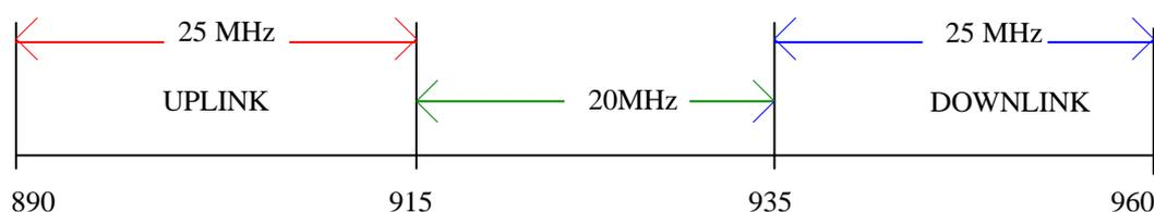
*Figure C1: The Uplink and Downlink bandwidths for GSM.*
