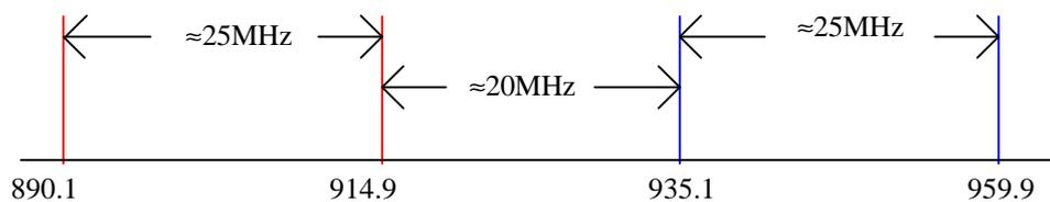
Figure C4: Selected channels spread over the bandwidth.
